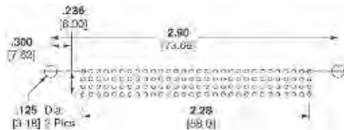
Recommended PC Board Layout for 1375797-1, 1375797-4, 1375798-1, 1375798-4
