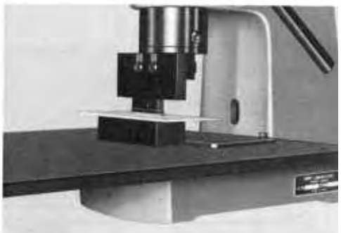
4. By pressing Mini-Press handle down, rest the press-fit jig against connector.
