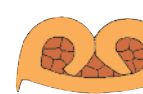
Flash at under side of crimp, due to over crimping Gratbildung am Crimpboden durch Überpressung
