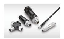
These **connector systems** provide an ideal solution for sensors and actuators in many industries. binder offers connectors from IP40 to IP69K, many with UL, VDE and Ecolab approvals, as well as FDA-compliant models. Users can order circular connectors with 2 to 12 contacts and a variety of termination options, including solder, crimp, dip solder, wire and twisted. M5, M8 and M12 screw-locking connectors are available in straight, right-angle and flanged styles.
